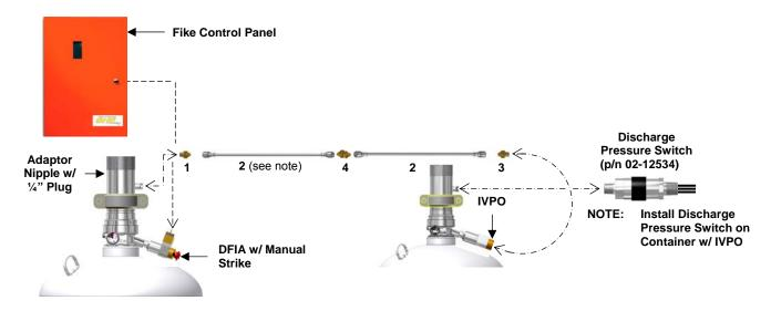
$1^{st}$  remove the  $\frac{1}{4}$ " NPT Plug from Adaptor Nipple, then install Actuation System as shown above. Secure Actuation tubing to a solid surface. Anchoring into plaster, sheetrock wall or any other facing material is NOT acceptable. For additional information regarding the installation and resetting of the IVPO, refer to the IVPO Component Sheet (p/n 06-551).
