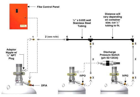
The illustration above shows the items required to make the proper connection between the Container equipped w/ an DFIA and the Container(s) equipped w/ an IVPO. The maximum length of pneumatic actuation line (including Hoses) can not exceed 50 ft. (15.2 m) and up to 6 containers equipped w/ an IVPO.
