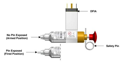
Install the wire lead w/ connector (Item no. 3) to the DFIA (Item no. 1) connector and secure with set screw.
